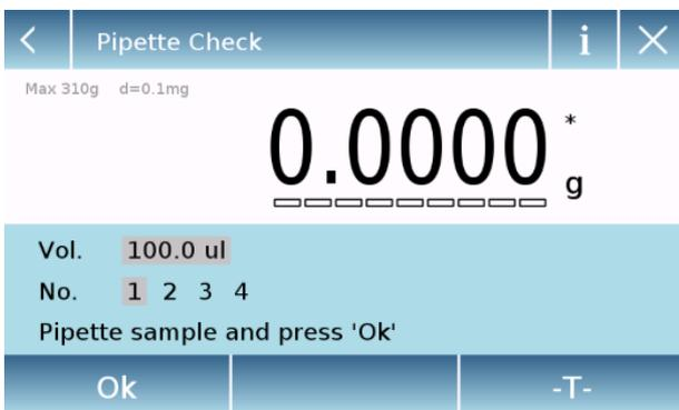
Then the pipette test begins. The number of weighs and the relative volumes vary according to the verification method selected and the type of pipette.
