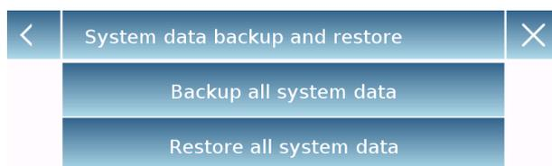
You can back up the system completely or restore data and configuration previously saved on a USB pen.
