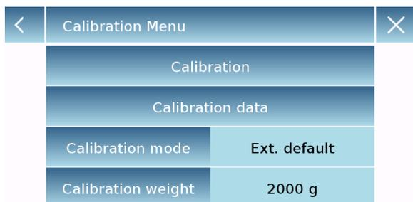
In the calibration menu, you can calibrate, display and print the data for the last calibration and set the calibration mode.
