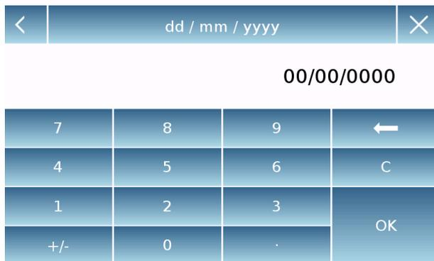
A numeric keypad will be displayed for entering the date and time in “**dd/mm/yyyy**” mode for the date and “**hh:mm:ss**” for the time
