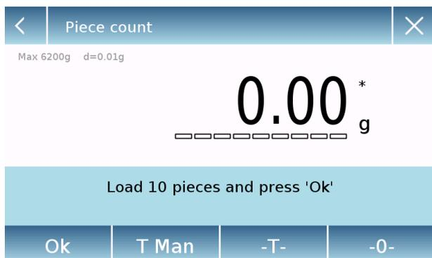
Do the tare of the container if necessary. In the case of sample counting, before counting it will be required to load the number of pieces chosen (for sampling) on the plate, while in the mode with average unit weight, you can start directly to count the pieces.
