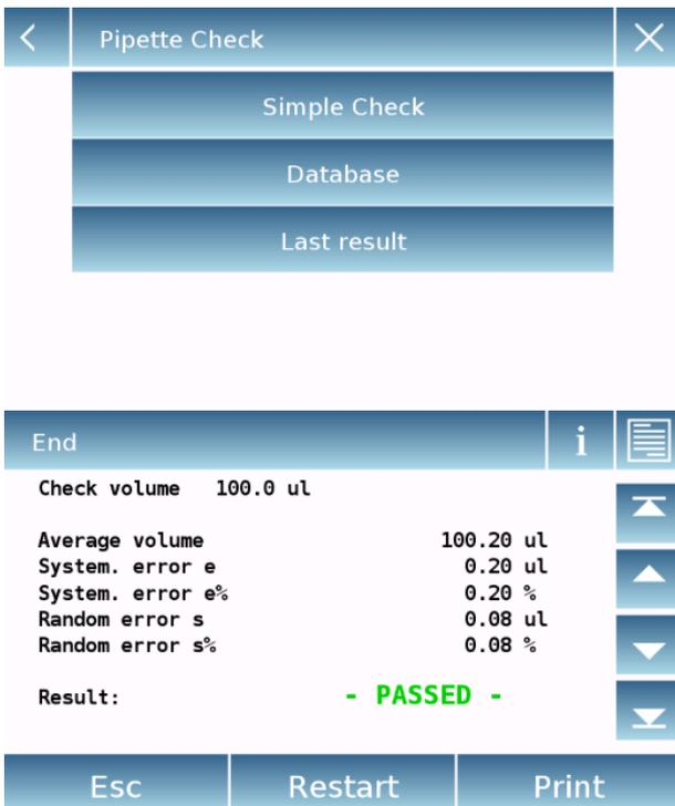
From the initial menu screen of the "pipette control function" by touching the "Last result" key, you can view the result of the last test performed.
