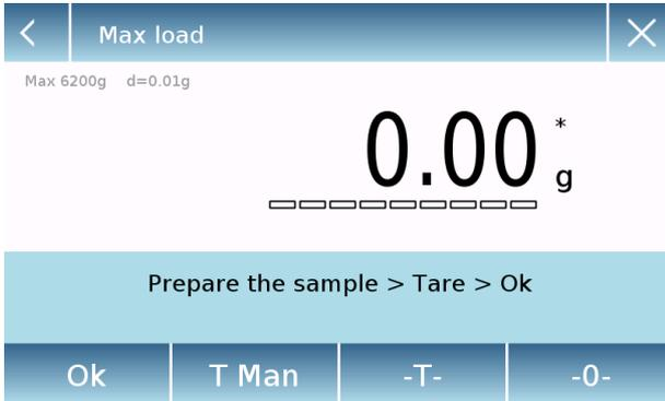
Selecting the function immediately displays the measurement screen.
