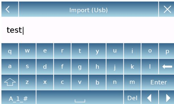
If the USB pen is inserted correctly, after confirmation, the alphanumeric keypad will automatically be displayed for entering the name of the backup you want to restore.
