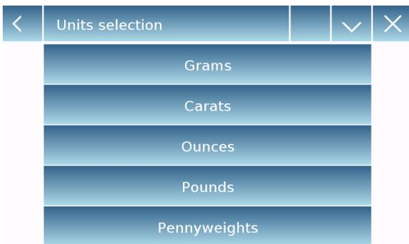
On the "**Units Selection**" screen, all available weighing units are immediately displayed. Touch the desired unit to enable it.
