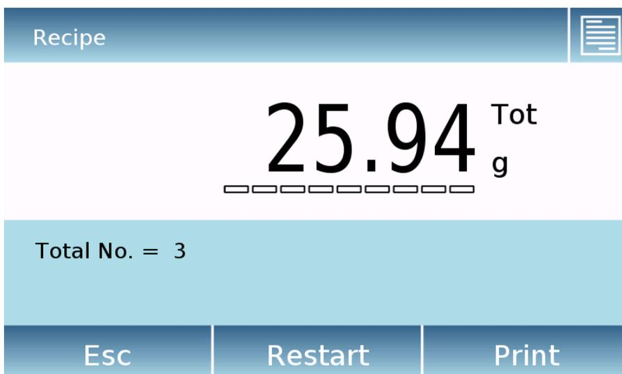
Touch the "Esc" key to exit the function, the "Restart" key to make a new measurement and the "Print" key to print the measurement result.
