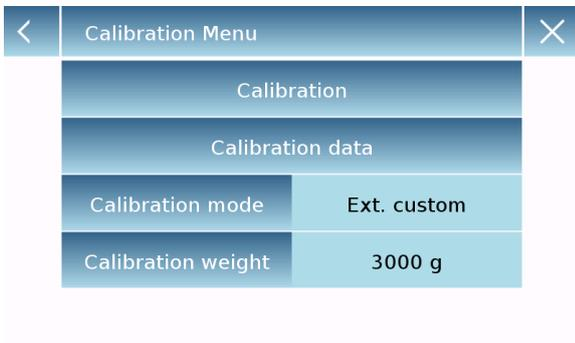
After selecting the "External custom", touch the weight setting key to set the desired weight value.
