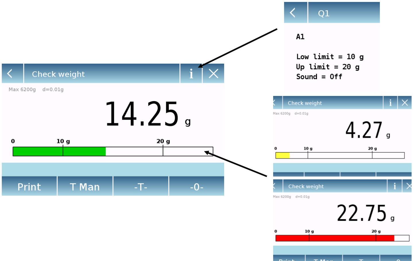
The Check weight bar is yellow when the loaded weight is lower than the minimum threshold and green when the weight is inside the set range (with the beep sound when activated) and red when the weight is greater than the upper threshold set.
