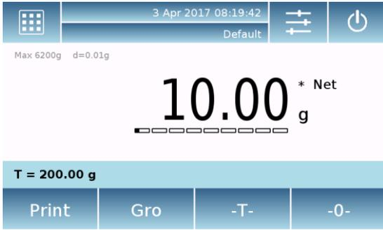
Place the sample to weight on the balance and wait for the stability symbol to light up before acquiring the value.
