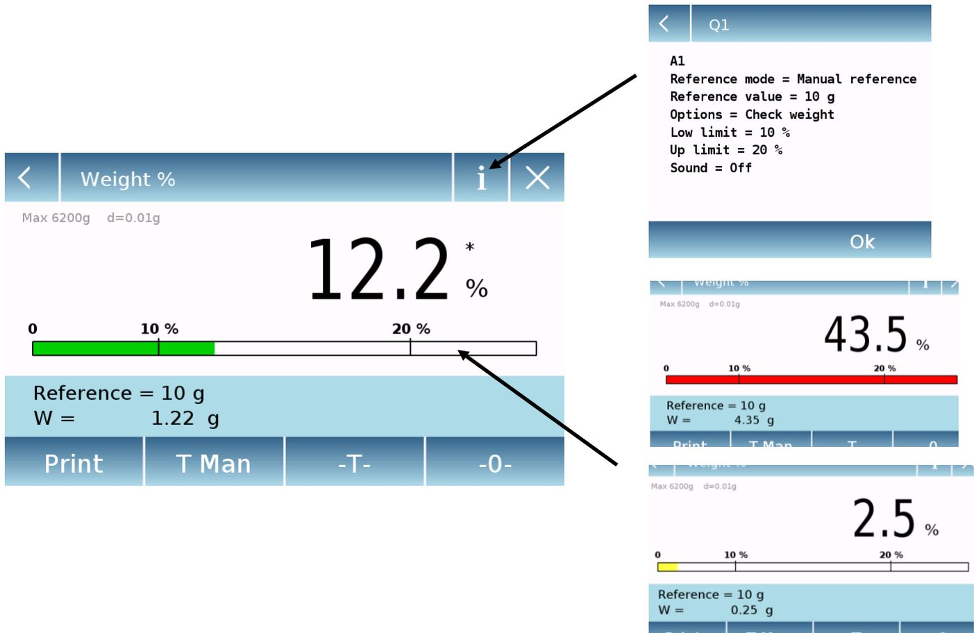
The weight check bar is yellow when the loaded weight is lower than the minimum threshold, green when the weight is within the set range (with the beeper when activated) and red when the weight is greater than the upper threshold set.
