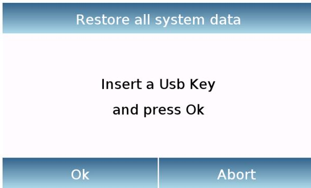
Insert the USB pen into the USB port on the left side of the balance, and press the "OK" key.
