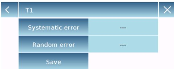
After entering the desired error values, touch the save button to confirm the settings.
