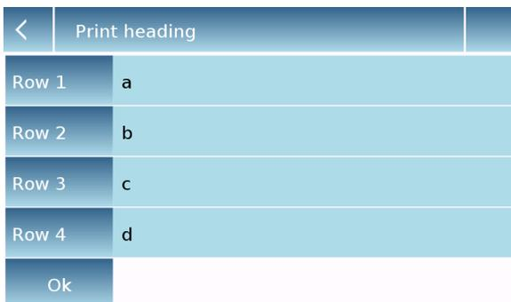
In the print heading screen, touch the areas that indicate the row number to automatically enable the alphanumeric keypad and enter the desired text with a maximum number of 40 characters per line.
