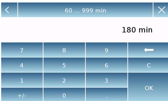
To change the auto-calibration range, touch the "Interval time" key and set the desired range between 60 and 999 minutes.
