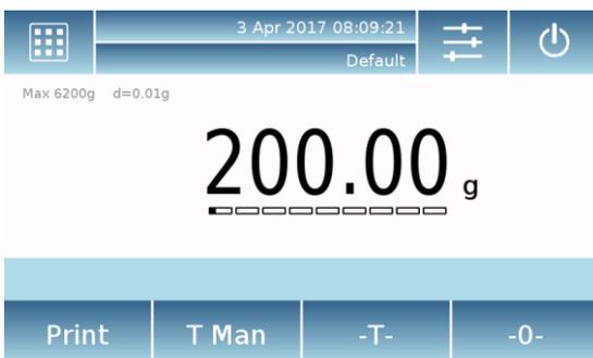
If you work with weighing containers, first zero the balance. Place the container and touch the **"-T-"** key.
