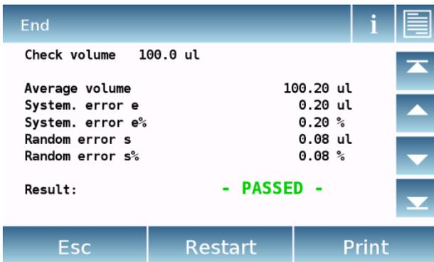
After the acquisition of the last value, a summary screen with the test results will be displayed.
