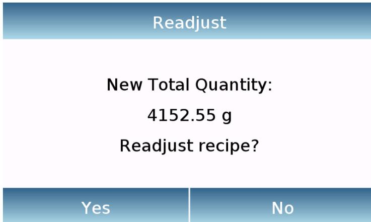
Touch the "Yes" key to confirm the adjustment, press the "No" key to return to the dosing screen. In this case, you can remove excess quantity or cancel the recipe by touching the "X" key.
