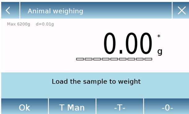
If necessary, reset the indication or load a tare.
