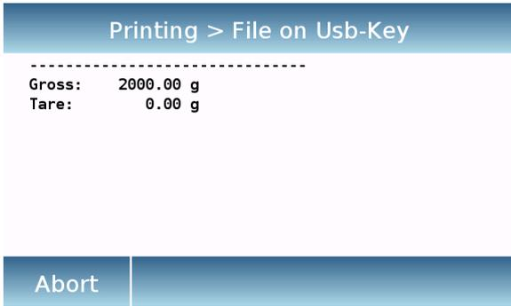
➤ **File on Usb-Key:** command print by touching the "Print" key will print to a file. In order to use this mode, you will need a USB pen to save the files. With the "File on Usb\_Key" mode enabled, before executing the print command verify that the USB pen is inserted in the USB port on the left side of the balance. While saving the file you can scroll on the screen through the information that will be saved in the file.
