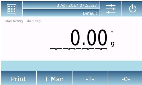
In the weighing screen, the area displaying the weight shows the value of the weight placed on the balance plate.
