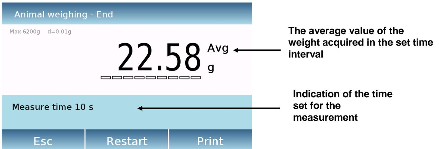
Touch the "**Esc**" key to exit the function, the "**Restart**" key to make a new measurement and the "**Print**" key to print the measurement result.
