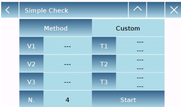
If the custom method is selected, it is possible to decide the number of weighs ("N"), the value of the volumes to be checked up to a maximum of three ("V") and the relative systematic and random error values.
