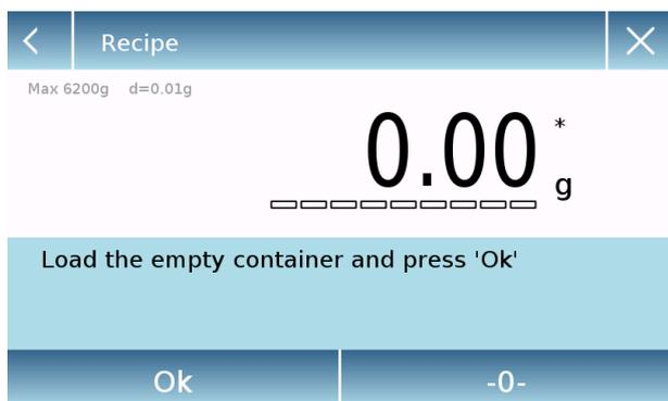
Touching the "Simple recipe" key immediately displays the measurement screen.
