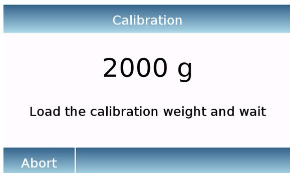
Load the required calibration weight or touch the "**Abort**" key to cancel the calibration procedure.
